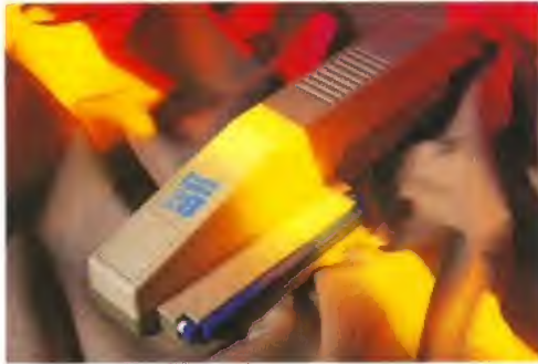
Supra's new Turbo 28 fits into the expansion slot on the A500, but includes a pass through port for hard disks.
